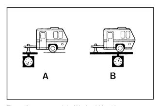
The trailer tongue weight (A) should be 10 percent to 15 percent of the total loaded trailer weight (B), up to a maximum of 400 lbs. (181 kg) with a weight carrying hitch. The trailer tongue weight (A) should be 10 percent to 15 percent of the total loaded trailer weight (A), up to a maximum of 900 lbs. (408 kg) for a weight distributing hitch.
